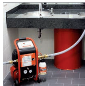
ROPULS with ROCLEAN Function: Flushing of drinking water pipes
