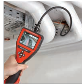
Inspection of hollow spaces
