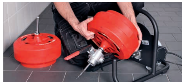
Interchangeable drum for different working ranges
